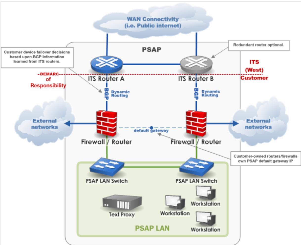
Figure 2: Host-Remote/Multi-node/ESInet Architecture
